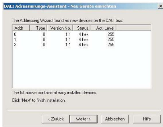
Then (!) search for additional new and unprogrammed devices, such as additional ballasts. If none are available, the previous list will be displayed.
