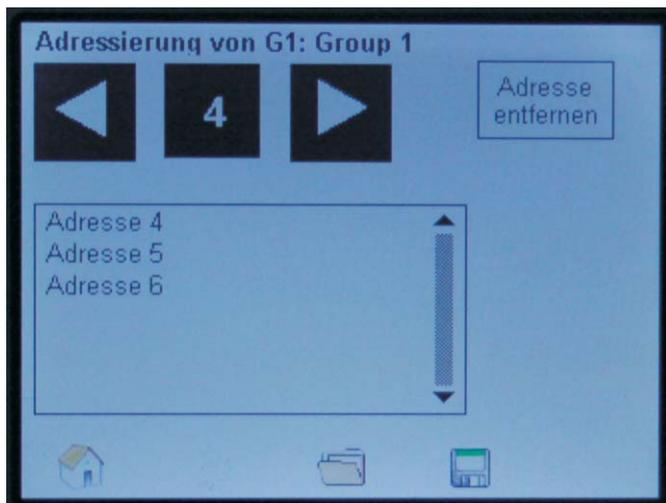
3. This is the result from the address search. Group assignments must be adjusted manually according to your system requirements. All groups are set by default.
