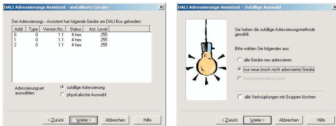
Devices on the bus are retrieved, example shows just one board 7703PWM set to DALI address 001. This will display three valid addresses then. (Note that software may display addresses 0...63 while users interpret these as 1...64 - this is due to the internal computer numbering system).
