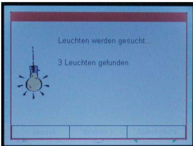
2. Attached devices are being detected. In this case, we have one 7703PWM attached set to start address 004. Thus, DALI addresses 4, 5 and 6 (3 addresses total) should be retrieved.
