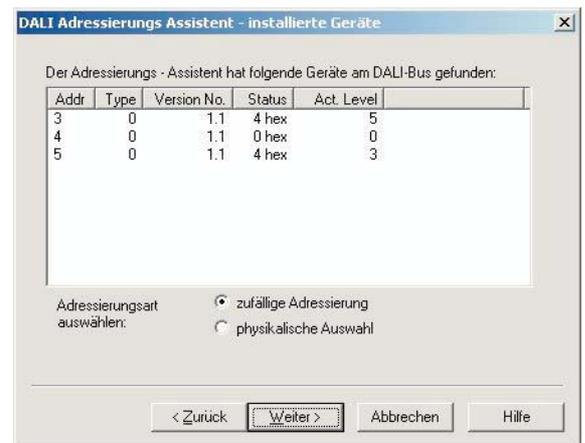
The last step will read the device properties. The 7703PWM will always be displayed as "DALI Ballast" with all groups assigned. Make changes as necessary to adjust for your system needs.
