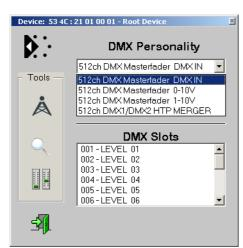
The DMX Multiplier 2101A-H complies to DMX RDM Standard 1.0. The unit must be configured via DMX RDM. The unit is recognized as signal processing device. It can be configured to four modes of operation using these DMX personalities:
