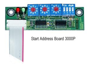
The 3000P can be replaced with the 3003P (LED display model).
