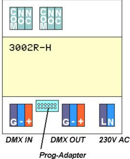
The drawing shows the position of the onboard connectors. Please refer to the text for functionality of the connectors.
