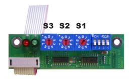
Setting address 000 will disable all outputs and sett all outputs to OFF regardless of data received.
