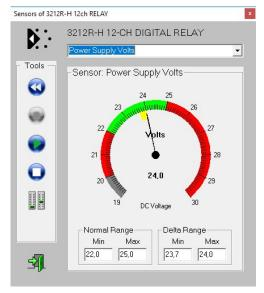
The 3212R-H consists of a integrated sensor for power supply monitoring.
