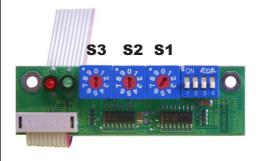
The three decimal coding switches set the start address, that is the address of the first channel to be decoded. The setting is fully decimal, no binary conversion is necessary as is with DIL switches.
