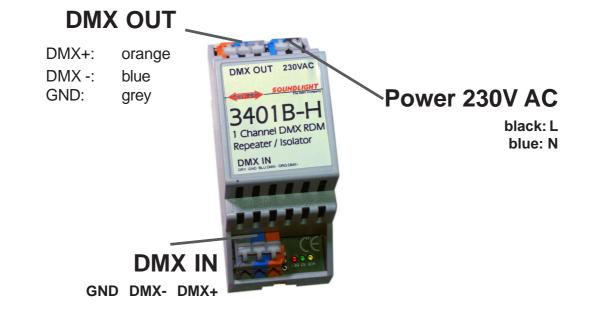
The 3401B-H is intended for 35mm standard DIN rail installation. Gently clip onto DIN rail. To unlock, use a screwdriver to pull yellow lever.
