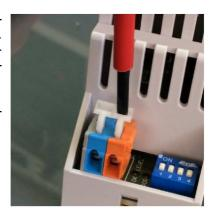
**DMX INPUT** Signal input for control signals according to USITT DMX512/1990 or DIN 56930-2
