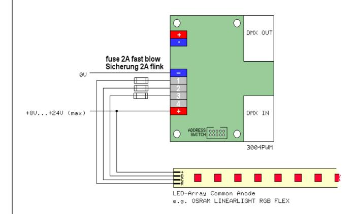
Driving voltage controlled LEDs using LED supply. Outputs must be fused externally 2A fast blow.
