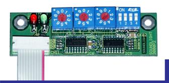
To program a DMX start address, simply set the desired start address. Wait some seconds until the unit recognizes and programs the address setting. The programming cycle will be indicated by the the red and green LED flashing alternatively four times.
