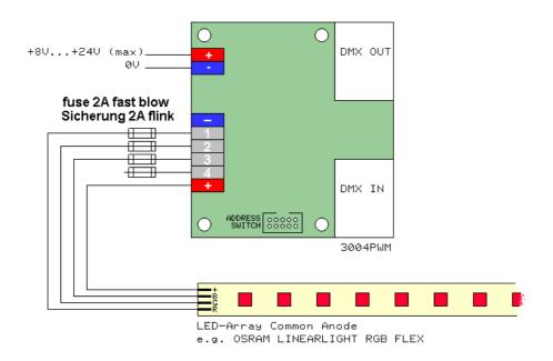
Driving voltage controlled LEDs, alternative supply method.
