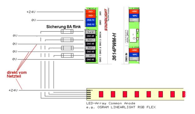
*Reference wiring scheme shown. The 3614 has four outputs; make sure that all GND terminals are wired to distribute current load. Use short wires of ample diameter to minimize voltage losses.*
