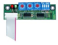
To program a DMX start address, simply set the desired start address. Wait some seconds until the unit recognizes and programs the address setting. The programming cycle will be indicated by the the red and green LED flashing alternatively four times.
