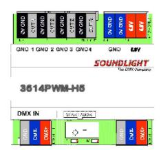
IMPORTANT NOTICE: Outputs are not short circuit protected and must be fused externally with appropriate fuse 8A fast blow.
