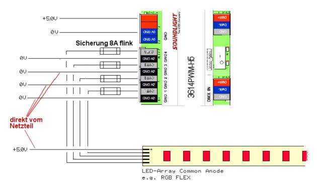
Reference wiring scheme shown. The 3614 has four outputs; make sure that all GND terminals are wired to distribute current load. Use short wires of ample diameters to minimize voltage losses.
