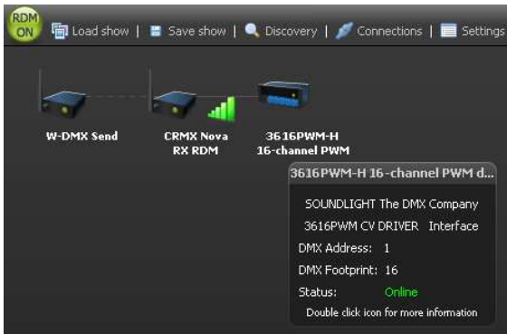
Recognizing the 3616PWM-H using Wireless DMX RDM (Screenshot: CRMX Nova Software)
