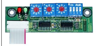
DMX Personality and DMX HOLD Options are set using the DIP switches onboard the 3000P2 start address board.
