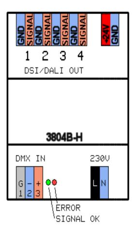
You may connect DSI (Digital Serial Interface) compatible or DALI (Digital Addressable Lighting Interface) compatible electronic ballasts (EVG) to the 3804B-H. Optimum performance will be obtained when using DSI compatible ballasts. The interface has to be programmed for DSI or DALI mode, see below. You are <u>not allowed</u> to mix DSI and DALI devices on one decoder.
