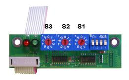
The start address can be set by DMX RDM using the START\_ADDRESS command (PID \$00F0). The start address defines the address of the first data slot used by the decoder. Valid start address settings include start adresss 001 thru 512-(number of slots used).
