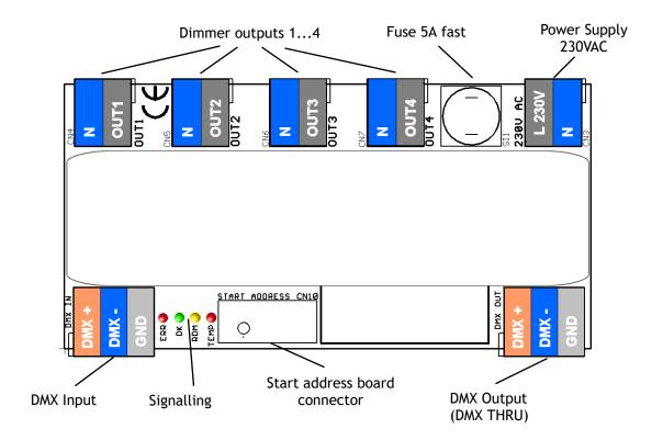
CN3 POWER SUPPLY 230V AC (cage clamp 2-polig)
