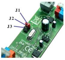
The decoder features internal jumpers to provide additional configuration of the unit. These settings are NOT for the standard user, they have been provided for technicians and experienced users to accommodate the unit to more sophisticated applications.
