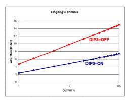
Input characteristics of the 1-10V to DALI converter 7601A-H
